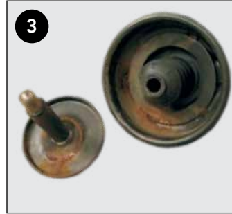
3 Damaged air chamber boots will cause water ingress to the caliper.
