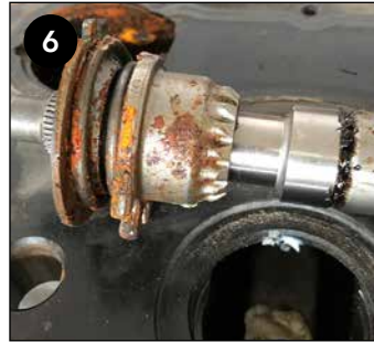
6 A major cause of caliper failure is due to water entry into the mechanism. 2ml of water is enough to prevent the caliper from functioning properly.
