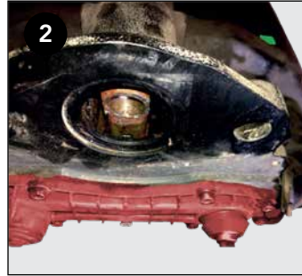
2 Check for rust on the lever of the caliper being replaced.
